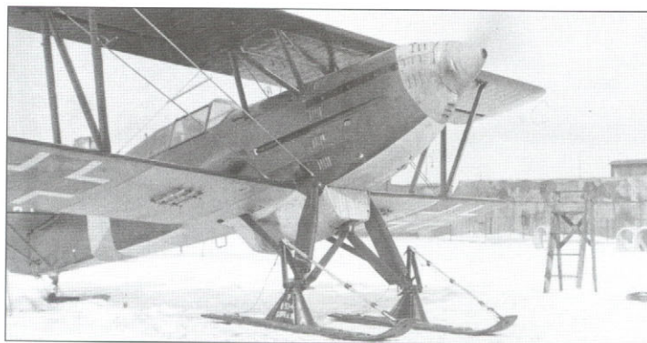
A cannon-armed Bk 534 fitted with Slovak-made skis has its engine run-up at Trencianske Biskupice aerodrome. Skis were used in field conditions only during 1942, when No 11 Sqn fought Soviet partisans in the Ukraine and Byelorussia
